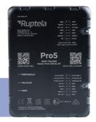
Advanced GPS tracker designed for all types of vehicles, including trucks, buses, and specialized machinery. It offers advanced capabilities such as reading on-board computer data (CAN), monitoring driver behavior, managing fuel, etc.
